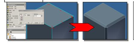
CHAMFER applies an angled edge; the size and angle can be varied.
