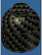
**Revolve** is a feature which is used to construct models which have more complex **PROFILES** such as curves, diagonals, etc.
