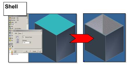
SHELL allows a solid object to be 'hollowed out'; the thickness of the walls being determined by the user.
