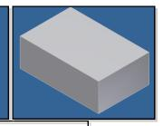
**Extrusion** is the most common feature used, and allows the construction of a 3D model with **VERTICAL SIDES**.
