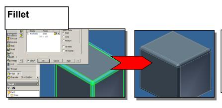
**FILLET** applies a **rounded edge** to the object; the size and style of the fillet can be varied.
