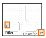
Rounds (fillets) corners; Angles (chamfers) corners
