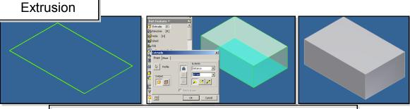
**Extrusion** is the most common feature used, and allows the construction of a 3D model with **VERTICAL SIDES**.
