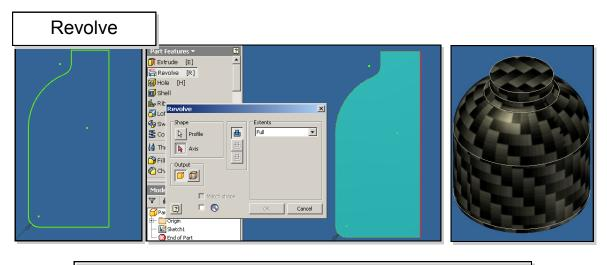
**Revolve** is a feature which is used to construct models which have more complex **PROFILES** such as curves, diagonals, etc.
